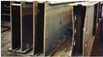
With hot-dip galvanisation, deformation of the structure is possible due to the use of high temperatures of molten Zinc. There is also potential for hydrogen embrittlement within welds.
